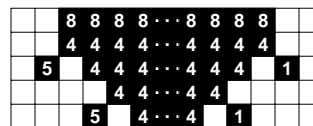
Figure 16. Evolution of long blocks of 4s and 8s in the domain filter output.
